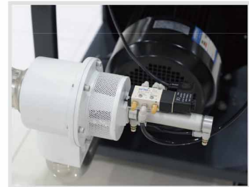
Vacuum breaking valve
